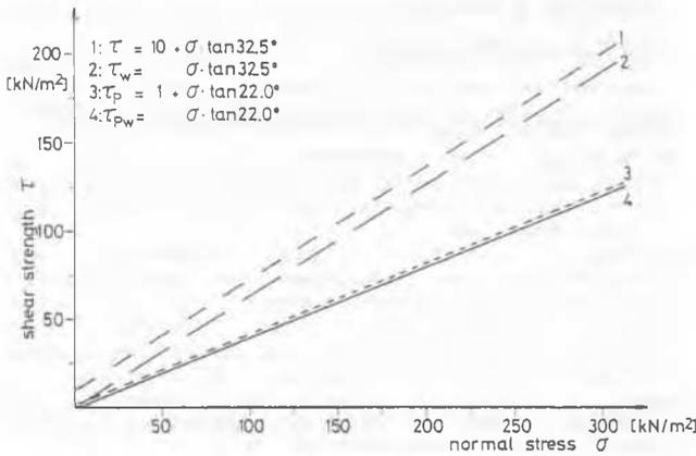
Fig. 5: Results of shear tests
