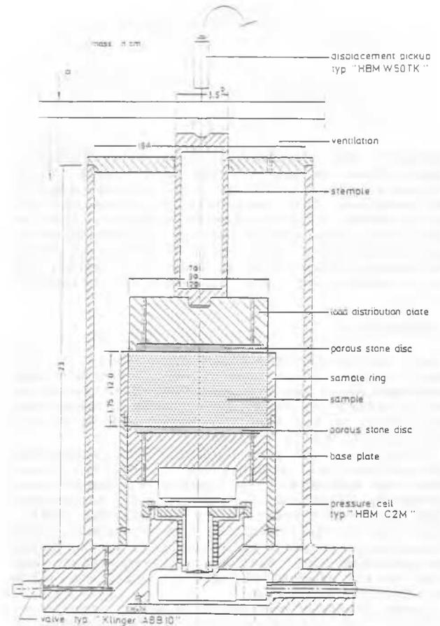
Fig. 4: Schematic section showing new developed oedometer
