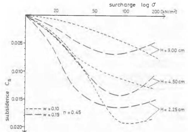
Fig. 7: Influence of water content (w), surcharge by wetting ( $\sigma_w$ ) and height of sample (H) for a constant porosity (n) and sample diameter (D = 4,5 cm) on the coefficient of subsidence ( $C_s$ )
