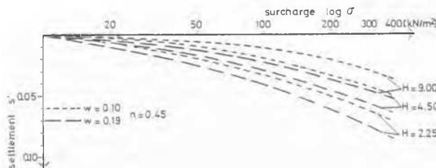
Fig. 6: Influence of water content (w) and height of sample (H in cm) for constant porosity (n) and sample diameter (D = 4,5 cm) on the settlement (s') of loess loam
