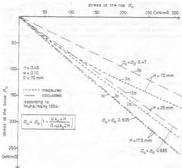
Fig. 8: Comparison of measured values by oedometer tests with those calculated by the formula of Muhs/Kany (1954)
