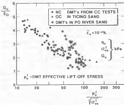
Figure 6. Evaluation of small strain shear modulus from DMT's for uncemented silica sands.
