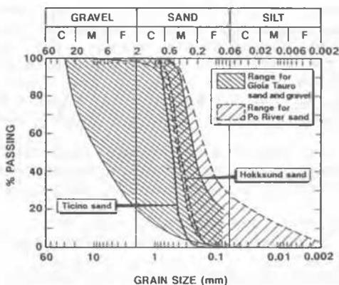
Figure 1. Granulometric characteristics of tested materials.
