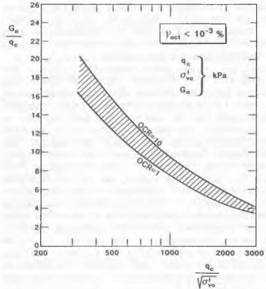
Figure 8. Evaluation of small strain shear modulus from CPT for uncemented silica sands.
