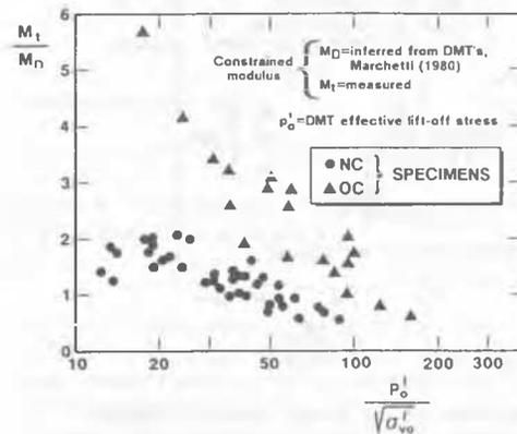
Figure 4. Constrained modulus of Ticino sand from DMT's performed in calibration chamber.
