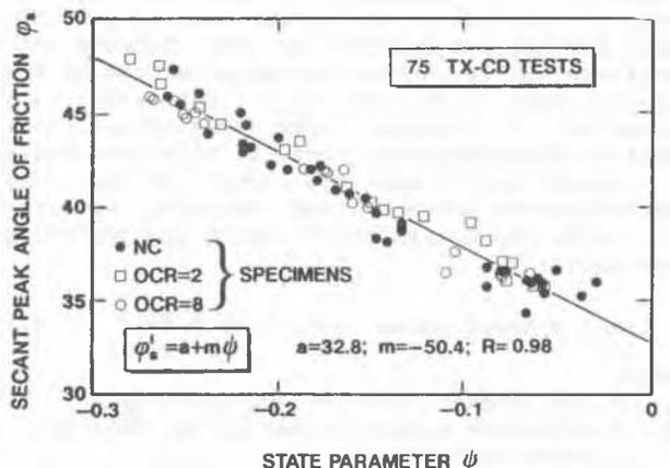
Figure 4. Friction angle of Hokksund sand vs. state parameter.
