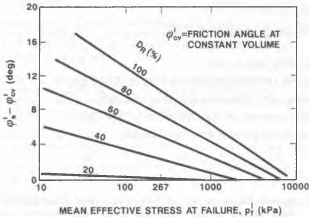
Figure 1. Generalized variation of triaxial peak  $\phi'_s$  with mean effective stress. After Bolton, 1986.
