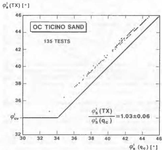
Figure 9.  $\phi'_S(q_c)$  for Ticino sand using Bolton's stress-dilatancy theory.
