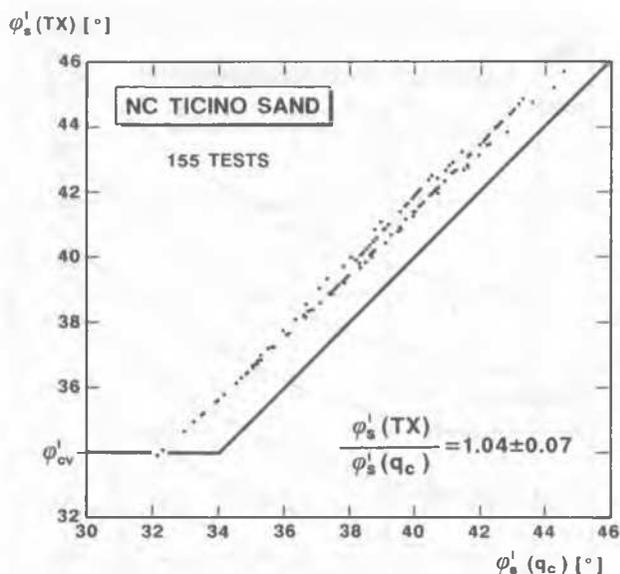
Figure 8.  $\phi'_S(q_c)$  for Ticino sand using Bolton's stress-dilatancy theory.
