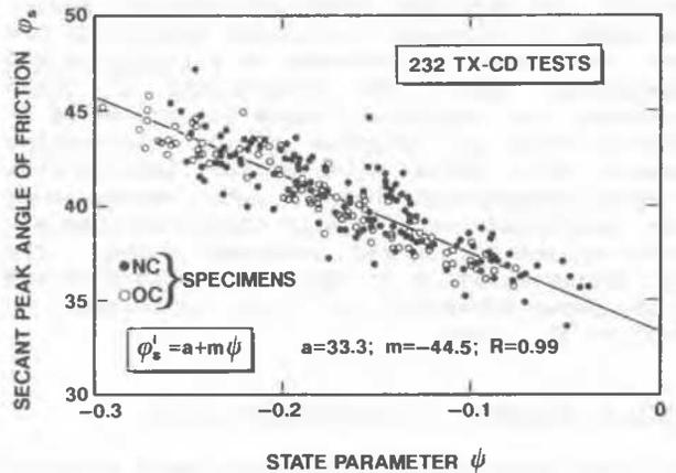
Figure 3. Friction angle of Ticino sand vs. state parameter.
