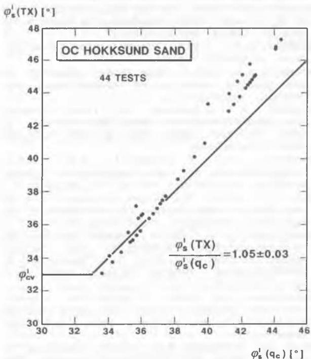
Figure 11.  $\phi'_s(q_c)$  for Hokksund sand using Bolton's stress dilatancy theory.
