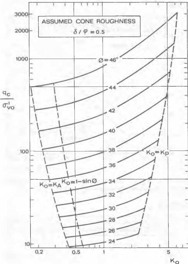
Figure 5. Chart for predicting peak friction angle ( $\phi'$ ) from CPT for uncemented, unaged, silica sands using Durgunoglu & Mitchell bearing capacity theory (Adapted from Marchetti, 1985).
