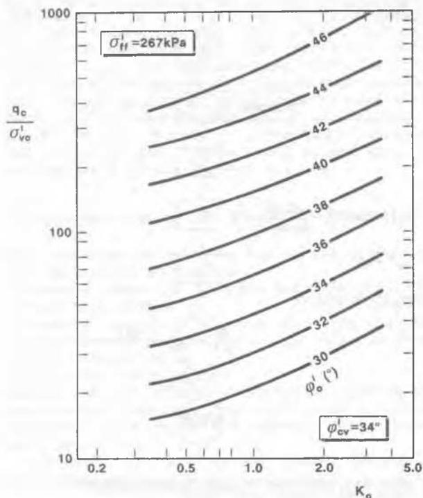
Figure 7. Friction angle  $\phi'_S$  of silica sand using Bolton (1986) stress-dilatancy theory. Adapted from Jamiolkowski et al., 1988.
