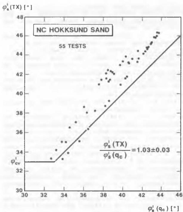
Figure 10.  $\phi'_s(q_c)$  for Hokksund sand using Bolton's stress dilatancy theory.
