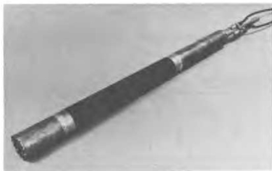
Figure 2. The weak rock self-boring pressuremeter.
