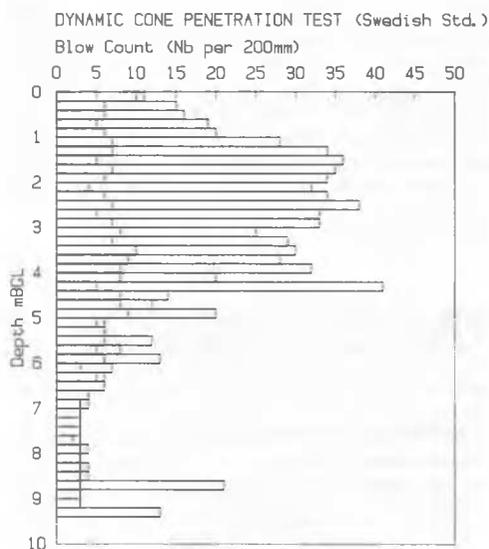
Figure 5. Dynamic penetration test results before and after vibroreplacement ground treatment.
