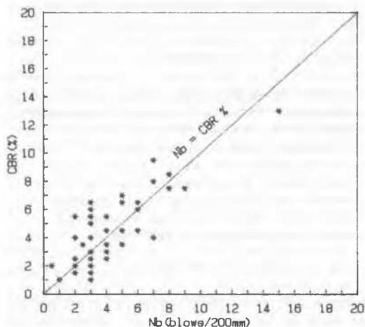
Figure 6. Correlation of dynamic penetration resistance with remoulded C.B.R. value (Road Note 29 Method).
