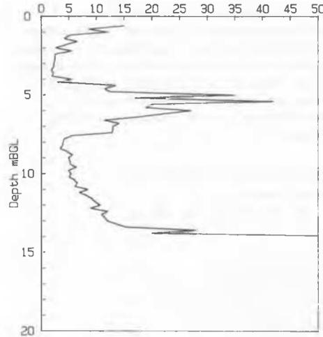
Figure 3. Result of static penetration test showing shallow and deep soft clay deposits.
