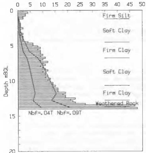
Figure 4. Result of dynamic penetration test at same location showing need for increased friction correction.
