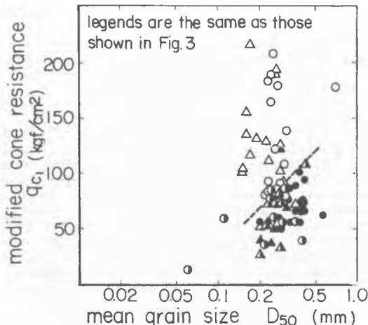
Fig. 4 Relationship between Mean Grain Size and Modified Cone Resistance for Liquefied Soil and No-liquefied Soils
