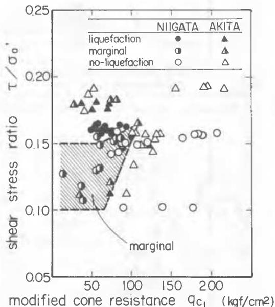
Fig. 3 Field Correlation between Shear Stress Ratio and Modified Cone Resistance  $q_{c1}$
