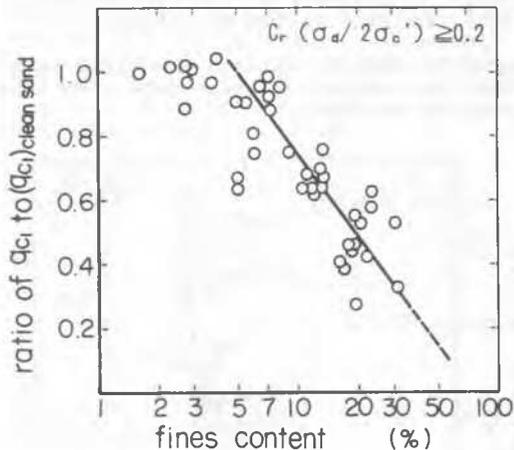
Fig. 9 Relationship between Fines Content and Ratio of Modified Cone Resistance for Equivalent Liquefaction Potential
