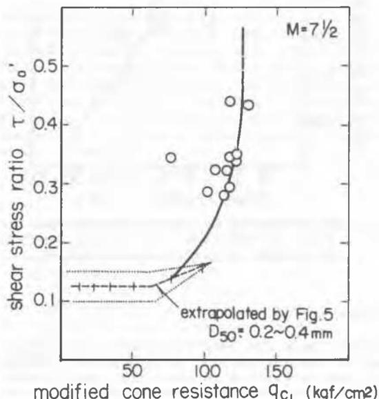
Fig. 8 Comparison of Laboratory Test Result and Field Correlation for Clean Sands (FC ≤ 5%)
