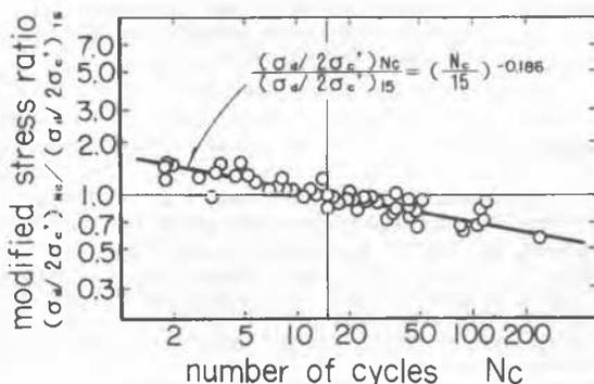
Fig. 6 Modified Cyclic Stress Ratio and Number of Cycles
