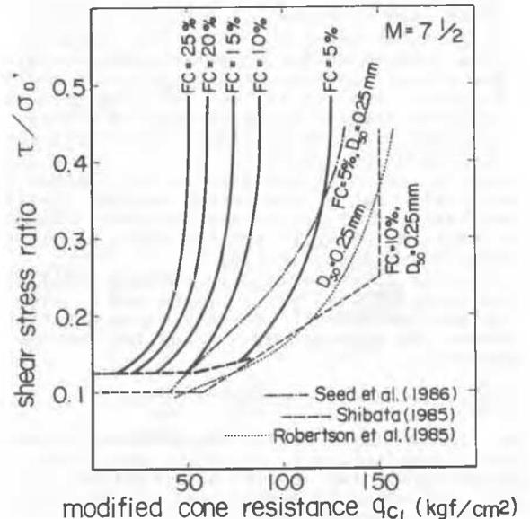
Fig. 10 Proposed Correlation between Liquefaction Resistance of Sands and Cone Resistance
