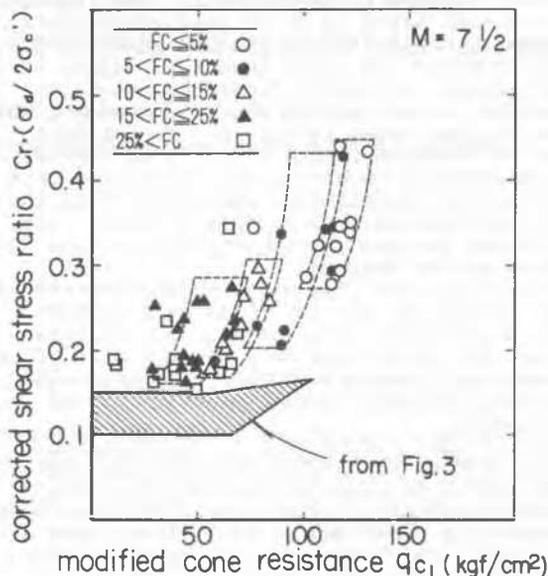
Fig. 7 Relationship between Stress Ratio Causing Liquefaction and Modified Cone Resistance Obtained by Laboratory Test
