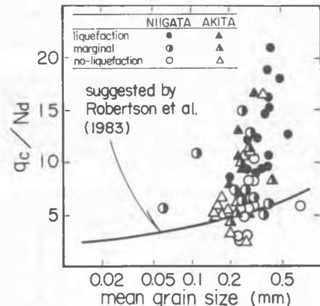
Fig. 1 Variation of  $q_c/N_d$  with Mean Grain Size
