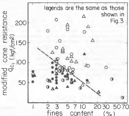
Fig. 5 Relationship between Fines Content and Modified Cone Resistance for Liquefied Soils and No-liquefied Soils
