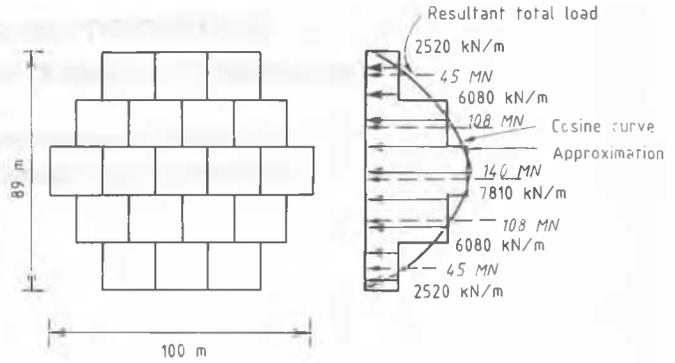
Figure 3. Step-function approximation of horizontal load.
