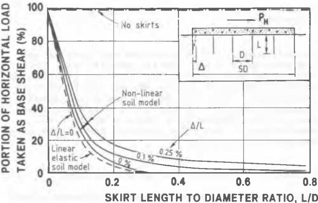
Figure 2. Shear on platform base due to horizontal load (Lacasse and D'Orazio, 1988).
