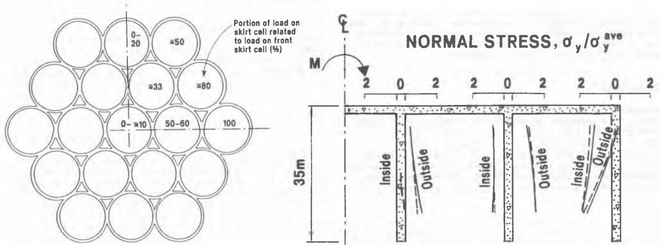
Figure 8. Theoretical stress distribution due to overturning moment (Lacasse and D'Orazio, 1988).
