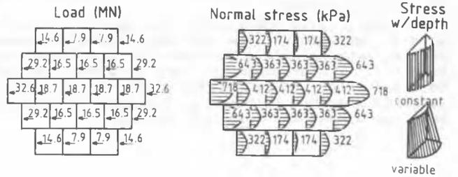
Figure 4. Load and stress distribution on each skirt due to horizontal load.
