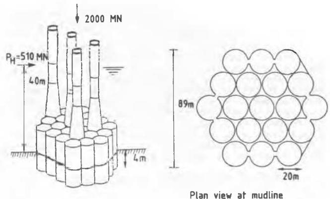
Figure 1. Sketch of platform and skirt configuration.
