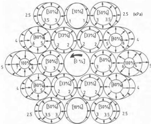
Figure 7. Stress distribution at  $d/L = 0.8$  due to overturning moment.
