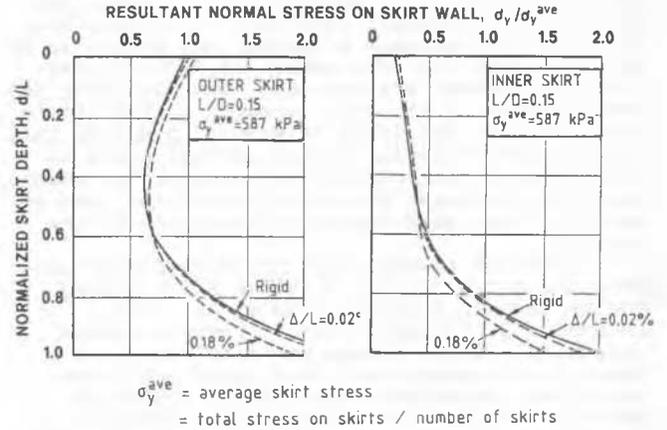
Figure 5. Stress distribution on skirts with depth due to horizontal load (Lacasse and D'Orazio, 1988).
