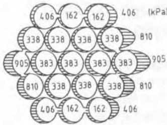
Figure 6. Stress distribution at  $d/L = 0.8$  due to horizontal load.
