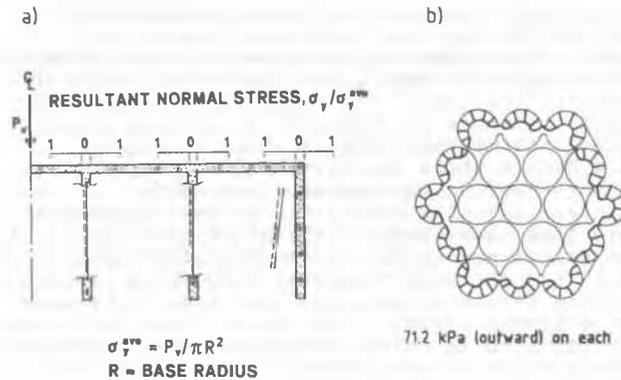
Figure 9. Stress distribution due to vertical load.
