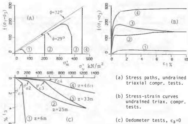
Figure 6. The soil parameters are determined from conventional triaxial and oedometer test results as reproduced above for the four layers of interest.
