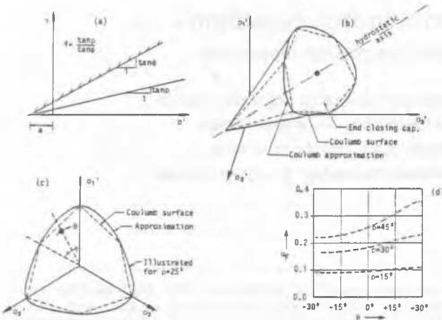
Figure 1. The yield criteria with: (a) definition of mobilized friction angle,  $\rho$ , (b) the cone and the plane cap in principal stress space, (c) the cone in the  $\pi$ -plane, (d) the  $\alpha_F$  coeff. of Eq.1a as a function of  $\theta$  and  $\rho$ .
