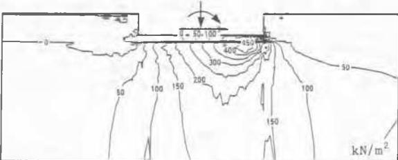
Figure 7c. Excess pore pressure for 1.3  $Q_h$  and 1.3 M
