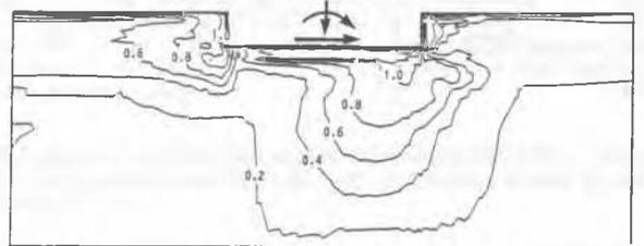
Figure 8b. Degree of mobilization for 3.0  $Q_h$  and 3.0 M
