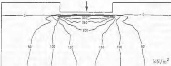
Figure 7b. Excess pore pressure after consolidation
