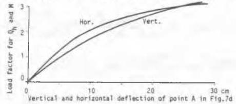
Figure 9. Load deflection curves for wave loading.
