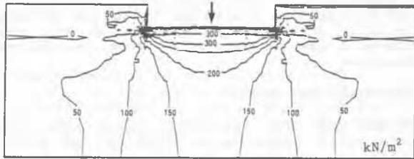
Figure 7a. Excess pore pressure from installation
