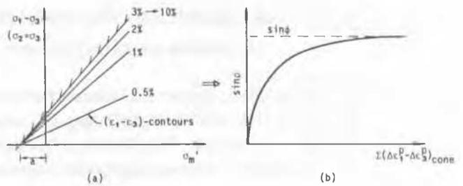
Figure 2. (a) Experimental findings indicate that the  $(\epsilon_1 - \epsilon_3)$ -contours are approximately straight lines. (b) Based on (a) we define a unique relationship between the mobilized friction and the plastic shear strains related to the Coulomb cone.
