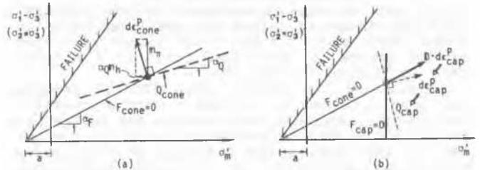
Figure 3. The plastic strain increments related to the cone (a), and the cap (b).
