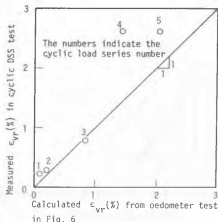
Fig. 7 Observed and calculated post-cyclic recompression volumetric strain in test (No. 7-2)
