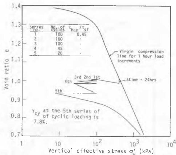
Fig. 5  $e$ - $\log \sigma'_v$  paths of O.C. clay with cyclic loading and drainage
