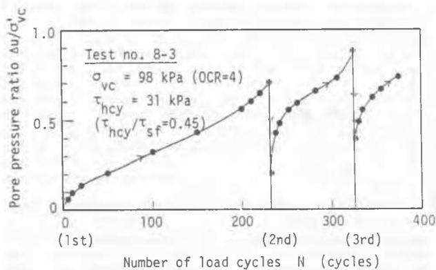
Fig. 3 Results from cyclic DSS test no. 8-3 with drainage
