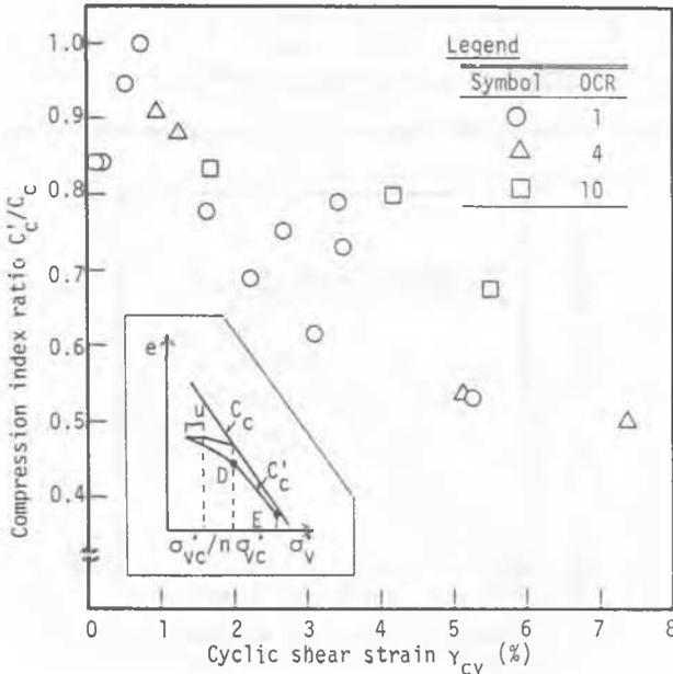
Fig. 9 Compression index in tests with cyclic loading with drainage
