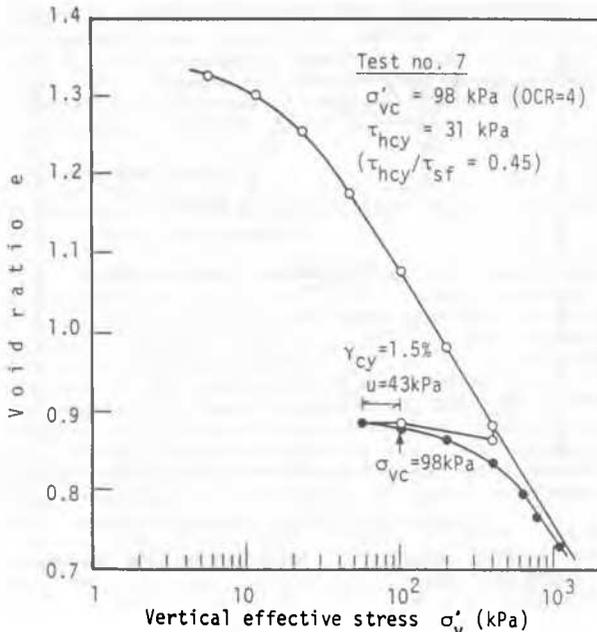
Fig. 8 e- log  $\sigma'_v$  relation for test with one series of cyclic loading with drainage
