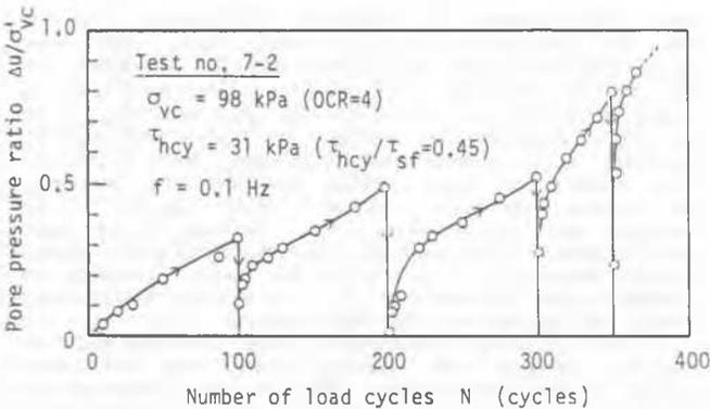
Fig. 2 Results from cyclic DSS test no. 7-2 with drainage
