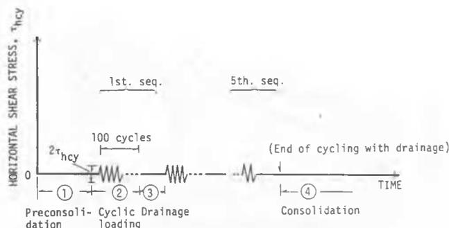
Fig. 1 Loading sequences of cyclic DSS test with drainage
