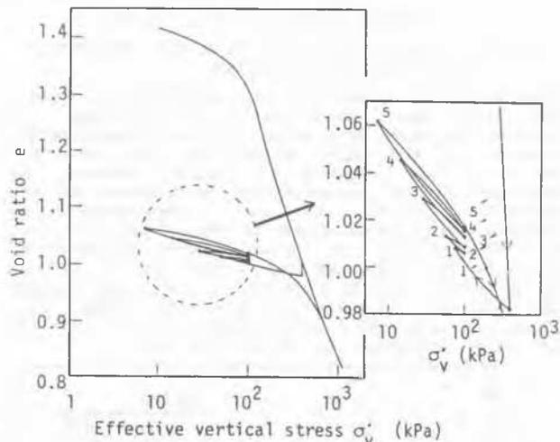
Fig. 6  $e$ - $\log \sigma'_v$  relations of O.C. clay in oedometer test
