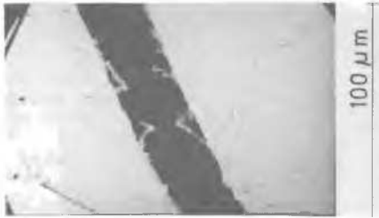
Figure 11. Possible formation of contact bonds between aggregates of Berkent bentonite, stored for 8 months /B/B-10g, 7%, 5000 RPM, 15 min/
