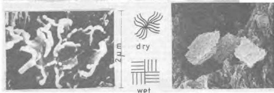
Figure 3. A cluster in Brebent bentonite. In wet state this cluster assumes a more regular form /B/R-2, 5%, 2000 RPM 5 min, unstored, dried at 20^\circ\text{C} /.
