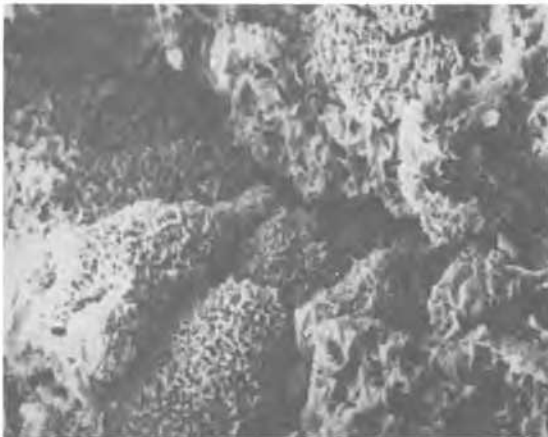
Figure 14. Deformation of an isotropic system in axial compression: bentonite from Zrecze Małe, compressed axially /a/, deformation of the structure /b/, stress - strain curves /c/.
