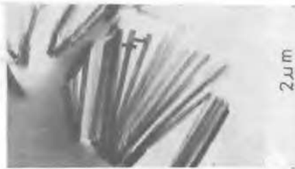
Figure 12. Uniformity of particle thickness after desintegration in microtome cutting /TEM, vermiculite, courtesy of H. Graf von Reichenbach/
