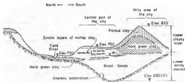
FIG. 1 - SKETCH OF A GEOLOGICAL SECTION OF SÃO PAULO TERTIARY BASIN
