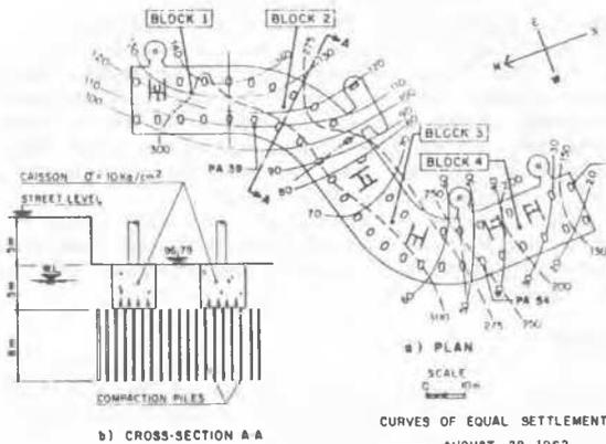
FIG 5 - COPAN BUILDING: FOUNDATION PLAN AND CROSS-SECTION, SHOWING CURVES OF EQUAL SETTLEMENT AT END OF CONSTRUCTION (AUGS. 28, 1962) AND RECENTLY (MARCH 5, 1988)
