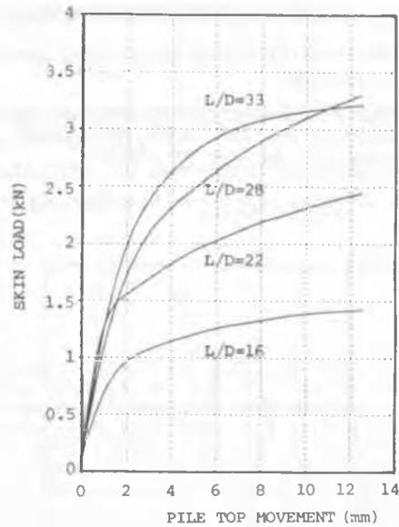
Figure 4. Skin load versus pile top movement for L/D ratios tested.
