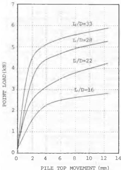
Figure 3. Point load versus pile top movement for L/D ratios tested.
