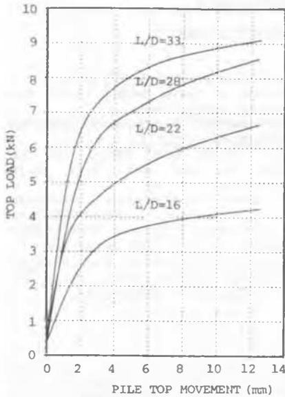
Figure 2. Top load versus pile top movement for L/D ratios tested.
