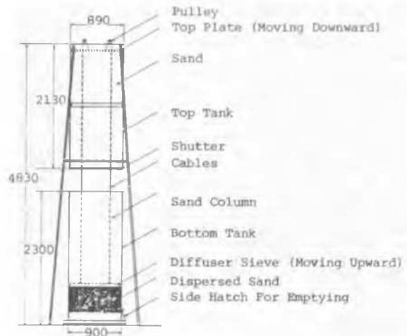
Figure 1. Schematic drawing of sand raining apparatus.
