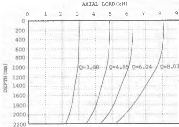
Figure 5. Axial load distribution for L/D=33.
