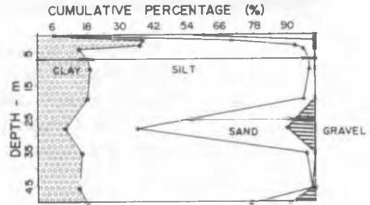
Fig. 4 Grain Size Distribution at a typical site
