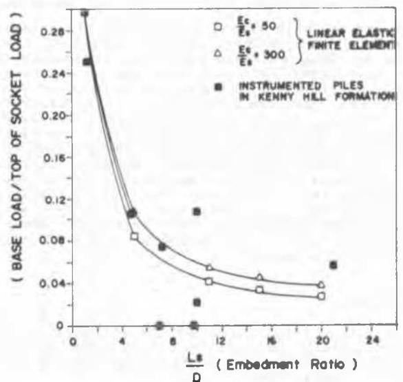
Fig. 10 Proportion of Base Load as a Function of Embedment Ratio
