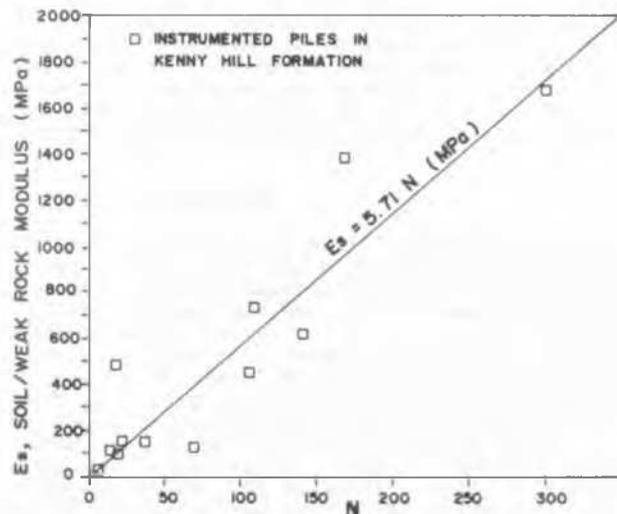
Fig. 9 Soil/Weak Rock Modulus versus N
