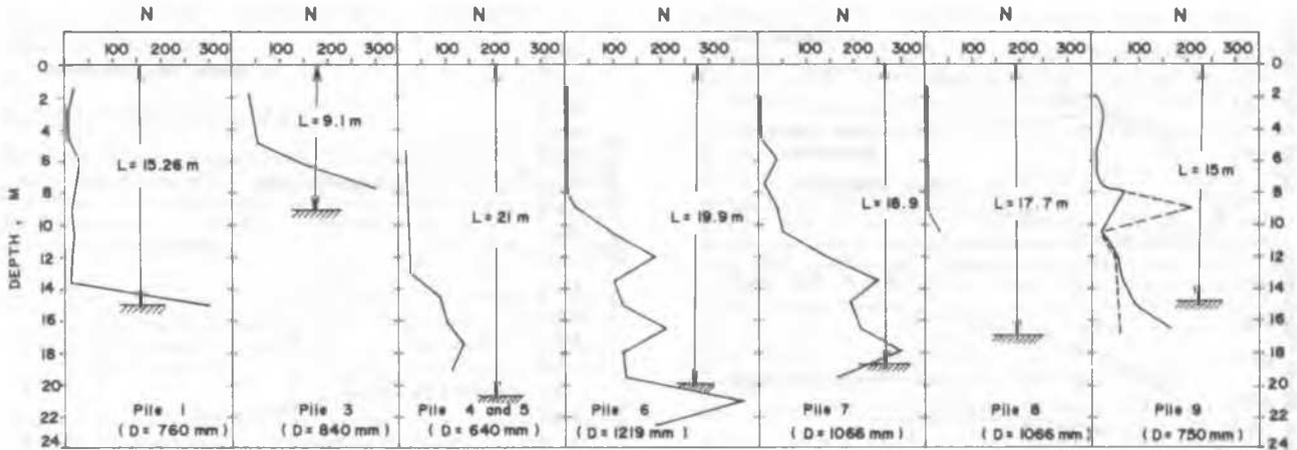
Fig. 5 Profiles of N and Pile Dimensions
