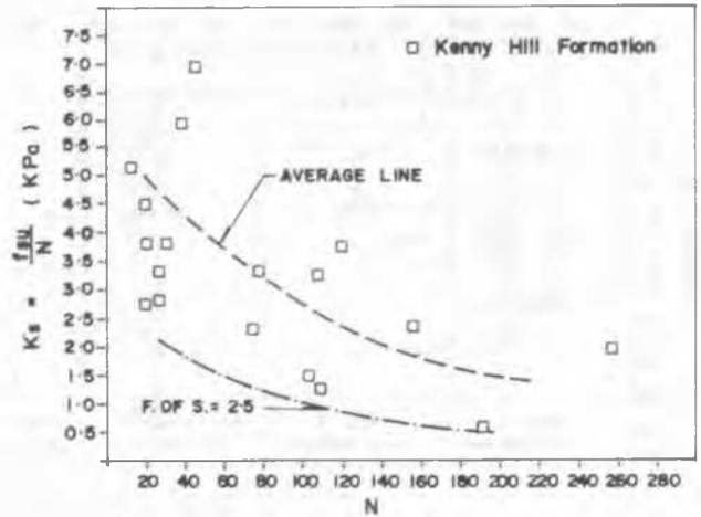
Fig. 7 Shaft Resistance Factor,  $K_s$ , versus  $N$
