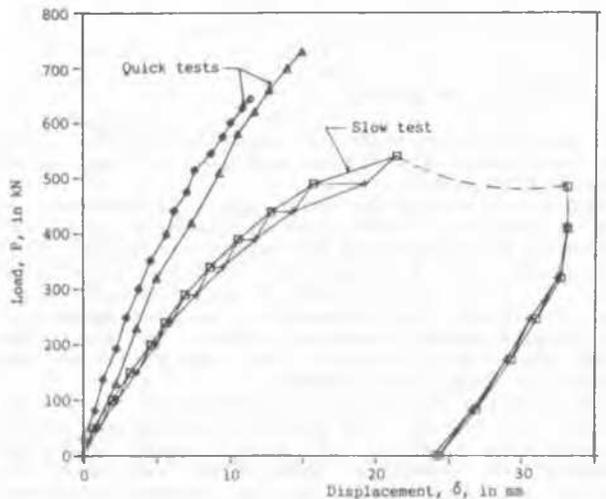
Fig 9. Slow and quick penetration tests
