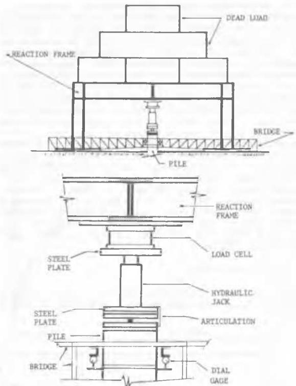
Fig 4. Loading system. Penetration test
