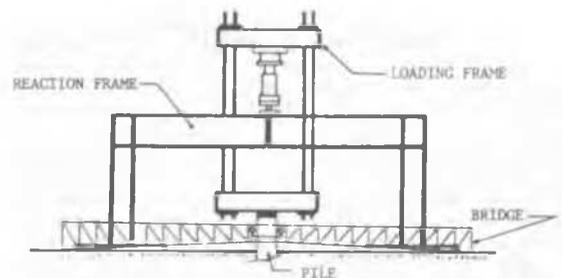
Fig 5. Pull-out loading system
