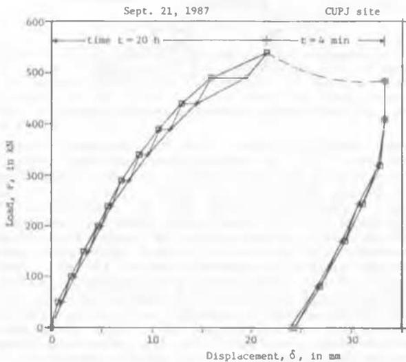
Fig 6. Slow penetration test
