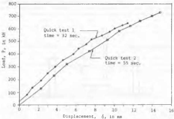
Fig 7. Quick penetration tests
