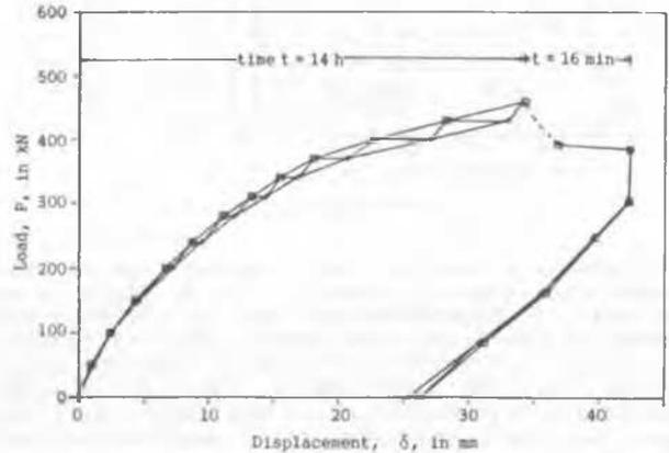
Fig 8. Pull-out test
