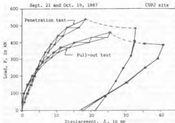
Fig 11. Corrected slow penetration and pull-out test curves
