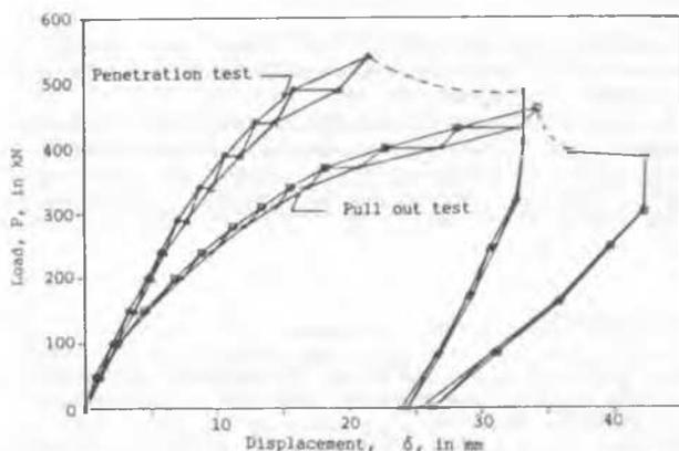
Fig 10. Slow penetration and pull-out tests
