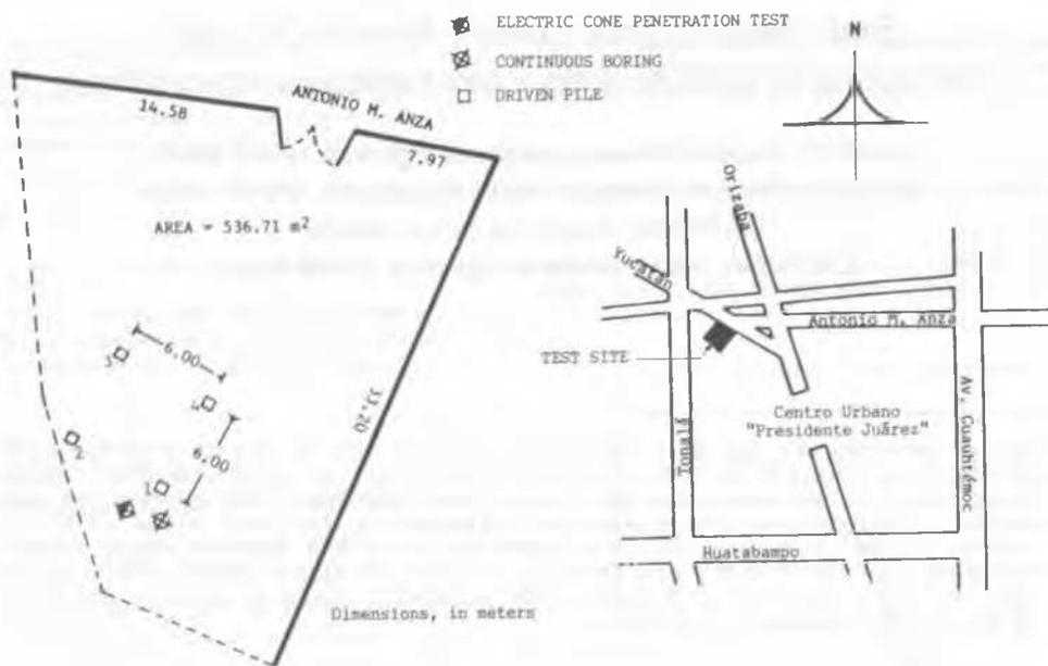
Fig 1. Site location, pile layout and borings
