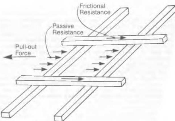
Fig. 1. Stress transfer between soil and reinforcement
