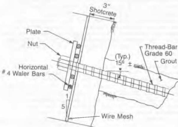
Fig. 4. Nailing details
