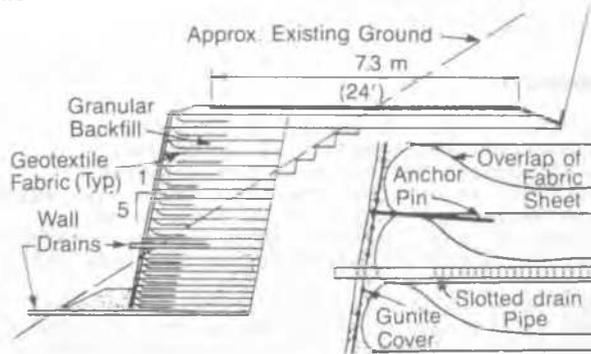
Fig. 2. Geotextile wall details
