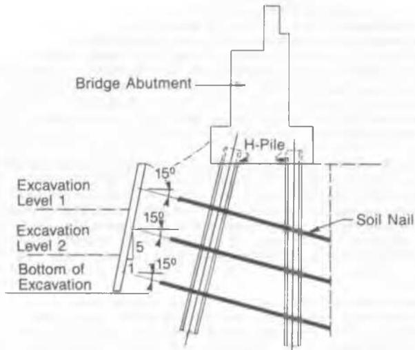
Fig. 3. Cross-section of nailed-soil wall
