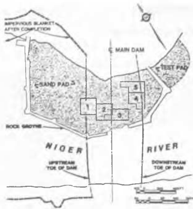
Fig. 2 Plan of Jebba Main Dam Area Showing Zones to be Densified by Deep Blasting
