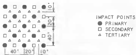
Figure 7. Typical Dynamic Compaction Grid Pattern
