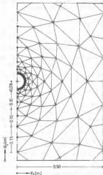
Figure 2. A symmetrical section of the FE mesh for the freezepipe system
