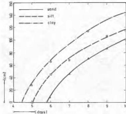
Figure 13. Progress of the frozen zone in days for sand, silt and clay
