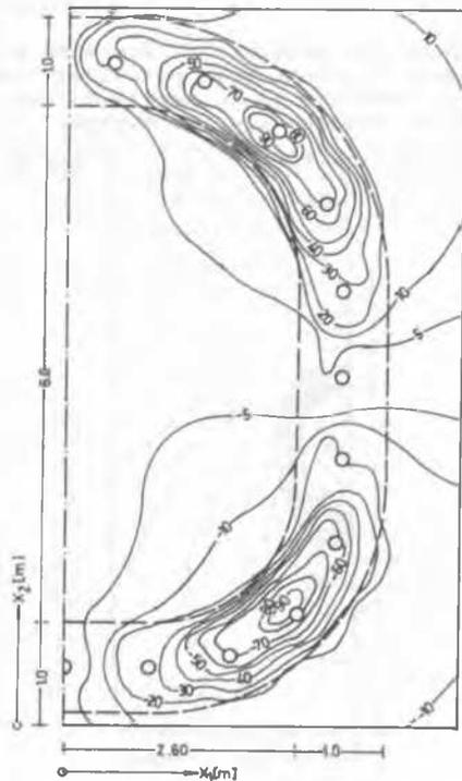
Figure 10. Isolines of shear stresses (kPa)
