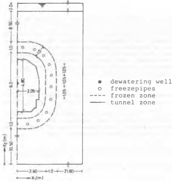
Figure 1. The freezing scheme using horizontal freezepipes
