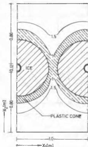
Figure 6. Isolines  $\tau_f/\tau$  in clays 5 days after freezing
