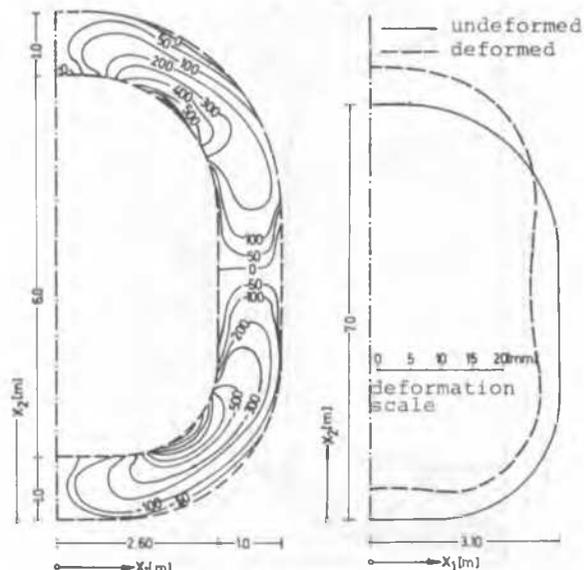
Figure 11. Isolines of shear stresses (kPa)
