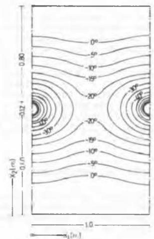
Figure 4. Isotherms after 10 days of freezing
