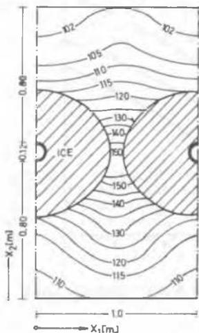
Figure 5. Isolines of excess pore pressures in clays 5 days after freezing (kPa)
