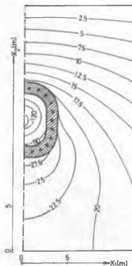
Figure 8. Excess pore-pressure isolines after freezing (kPa)
