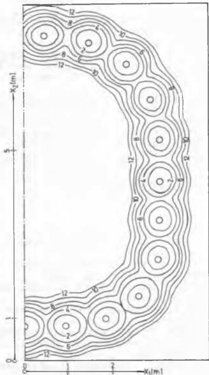
Figure 7. Progress of freezing in days
