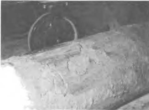
Figure 22. The surface of a pile after the load test.
