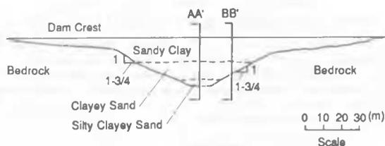
Fig. 1 Section along longitudinal axis looking downstream
