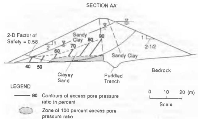
Fig. 4 Excess pore pressures in maximum cross section immediately after the earthquake
