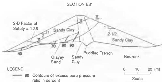
Fig. 5 Stability of typical abutment section immediately after the earthquake
