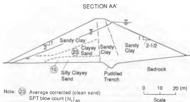
Fig. 2 Maximum cross section of dam
