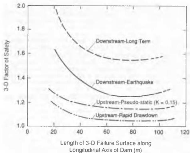
Fig. 6 Variation of 3-D factor of safety with length of failure surface
