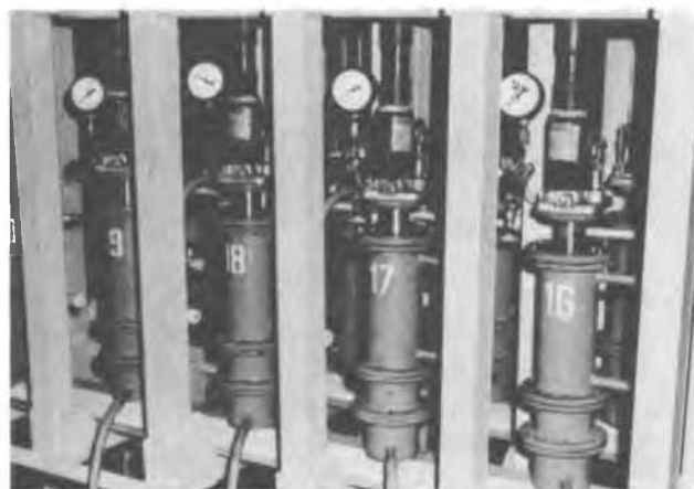
Fig. 1 - Apparatus for testing soil-geotextile interaction under high stress and high hydraulic gradients
