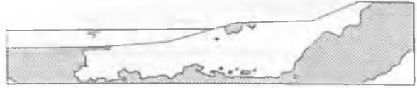
Fig. 4a. Plastic zone during failure of the Wolpherense Dike due to uplift.
