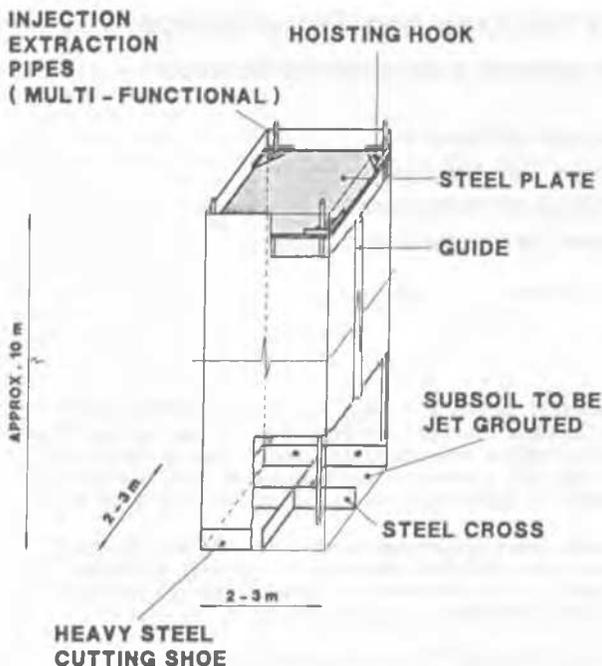
Figure 2. Example of a container-pile design
