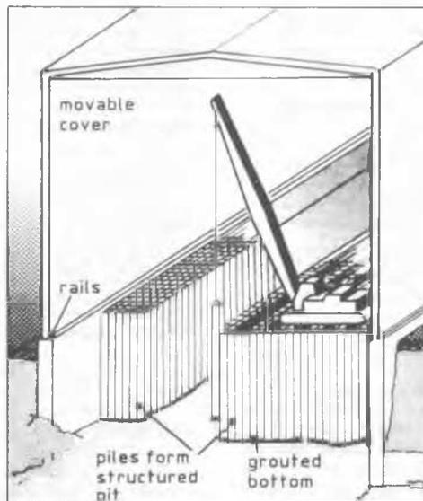
Figure 5. Example of a container-pile wash-installation
