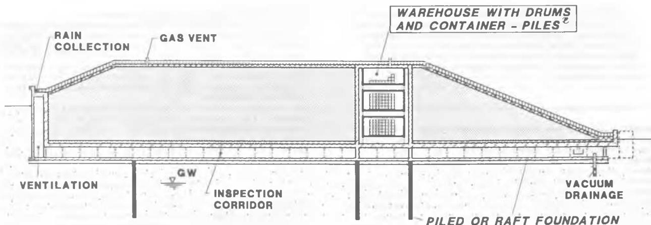
Figure 6.: Example of an inspectable controllable, safe, temporary storage facility
