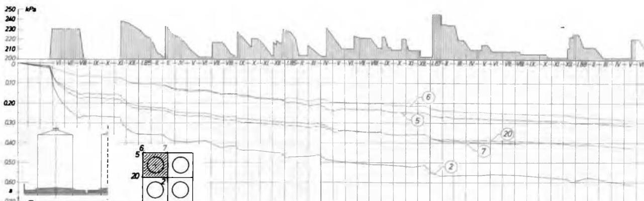
Figure 3. Observed settlements of one foundation slab of tank group II
