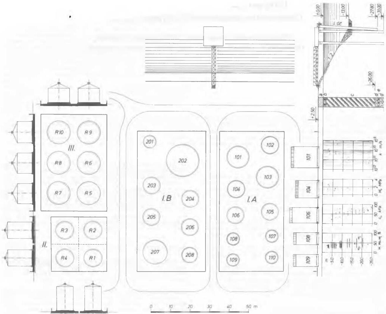
Figure 1. Site plan with cross-sections and geotechnical profile
