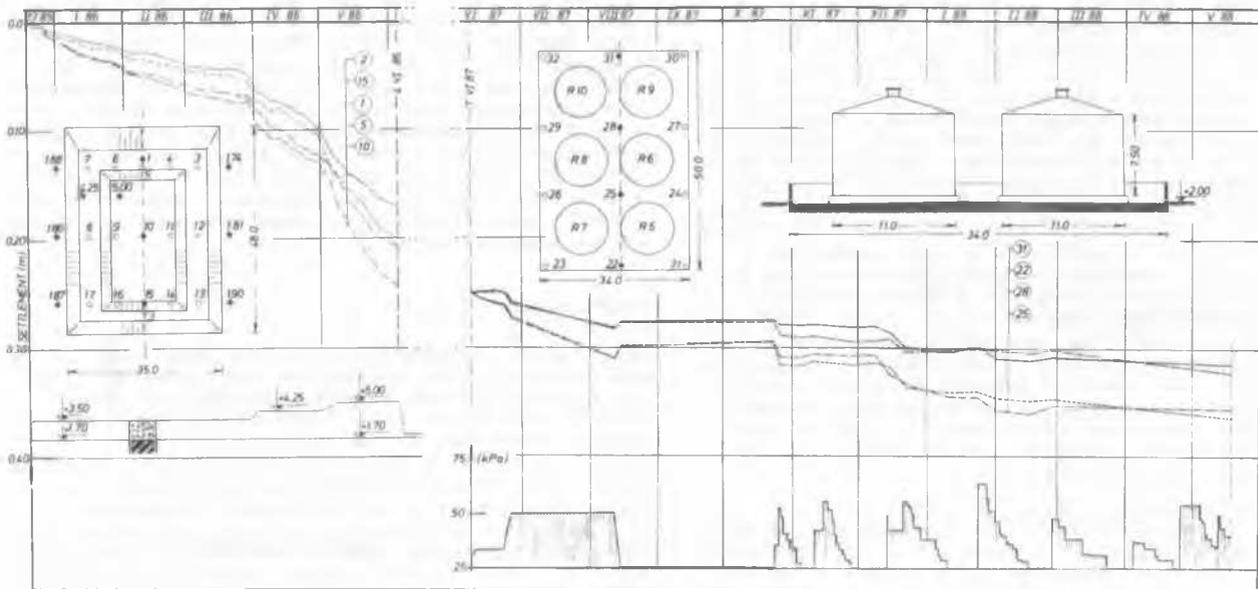
Figure 5. Observed settlements during preloading (left) and use (right) of tank group III
