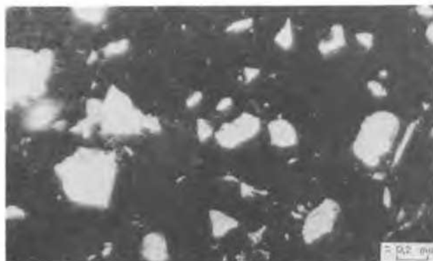
PLATE 4 - Residual soil of gneiss 2 m depth. Quartz grains ( \pm 30\% ), floating in a clay (mainly kaolinite) and iron oxide matrix ( \pm 70\% ).
