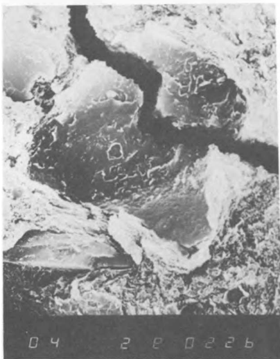
b) Scanning electron micrograph (2,000x) of a grain of parallel structure within the matrix of cluster structure (Brebent bentonite Na, picture breadth 50 \mu\text{m} )
