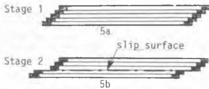
Fig. 5 Deformation of sample contained in tightly fitting rings without membrane.
