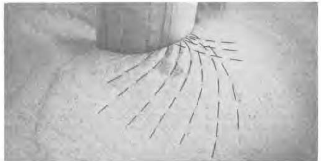
Fig. 3 Narrow rupture zone at the sand surface
