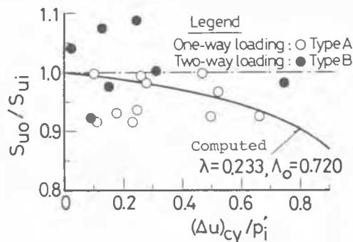
Fig. 7 Computed and Observed Undrain-Strength of Clay Samples after Undrained Cyclic Loading
