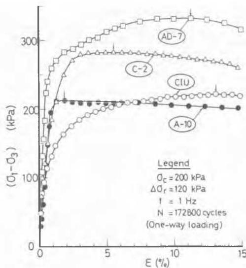
Fig. 6 A Comparison of Stress-Strain curve for Clay Samples after Cyclic Loading
