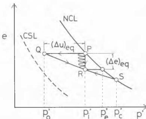
Fig. 8 Definitions of  $(\Delta u)_{eq}$  and  $(\Delta e)_{eq}$  during Drained Cyclic Loading
