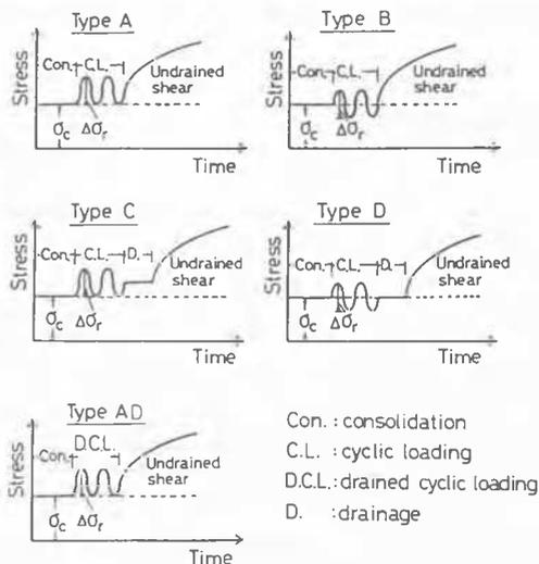
Fig. 3 Loading Sequence of Cyclic Tri-axial Compression Tests
