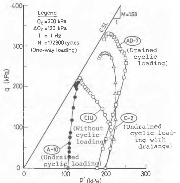
Fig. 4 A Comparison of Effective Stress Path of Clay Samples after Cyclic Loading
