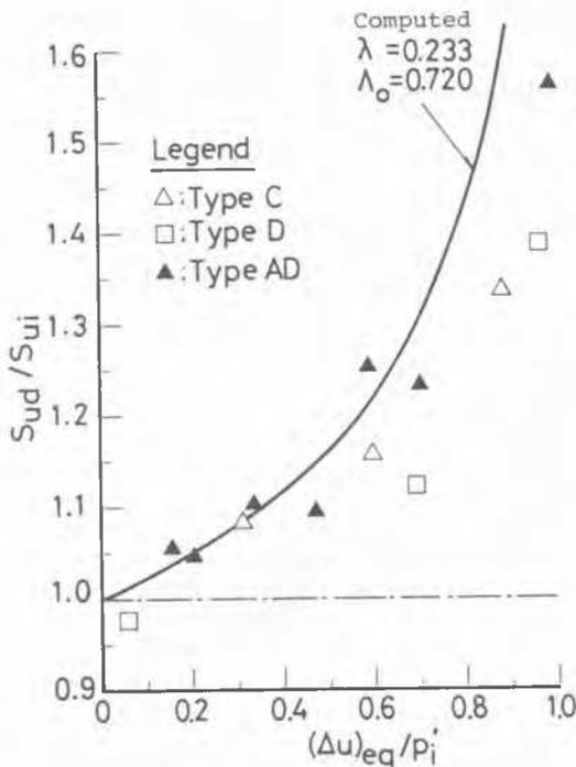
Fig. 9 Computed and Observed Undrained Strength of Clay samples after Undrained cyclic Loading with Drainage and Drained Cyclic Loading
