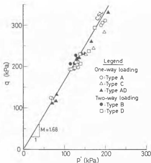
Fig. 5 End points of Effective Stress Paths for Clay Samples Failed under Cyclic Loading
