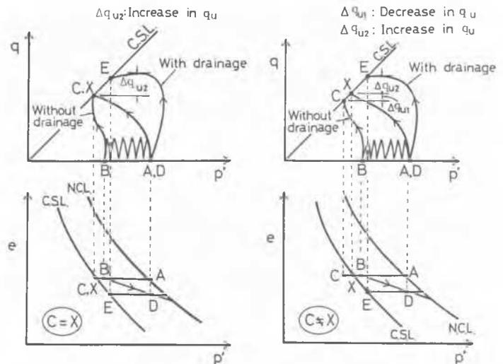
Fig. 1 Stress and State Paths after Cyclic Loading (Model A) Fig. 2 Stress and State Paths after Cyclic Loading (Model B)
