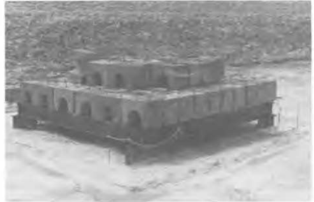
Figure 4: Photograph of Loading Frame
