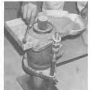
Fig. 3 Sectional Sampling Using Thin-Wall Rings
