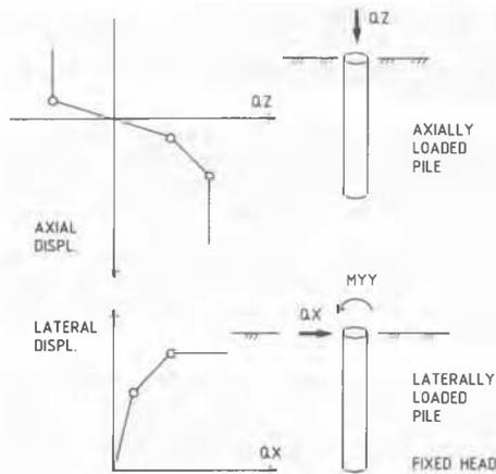
Fig. 6: Axial and Lateral Non-Linear Behaviour of Piles
