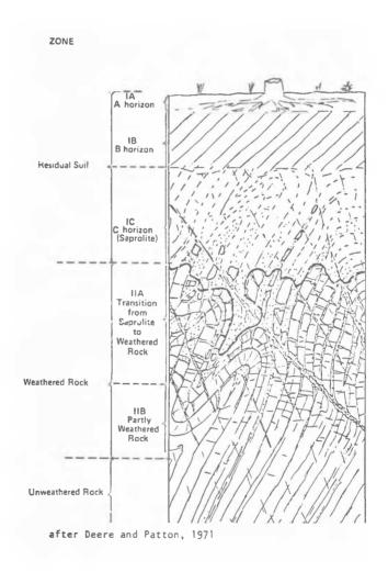
Fig. 1 Weathering Profile for Metamorphic Rocks
