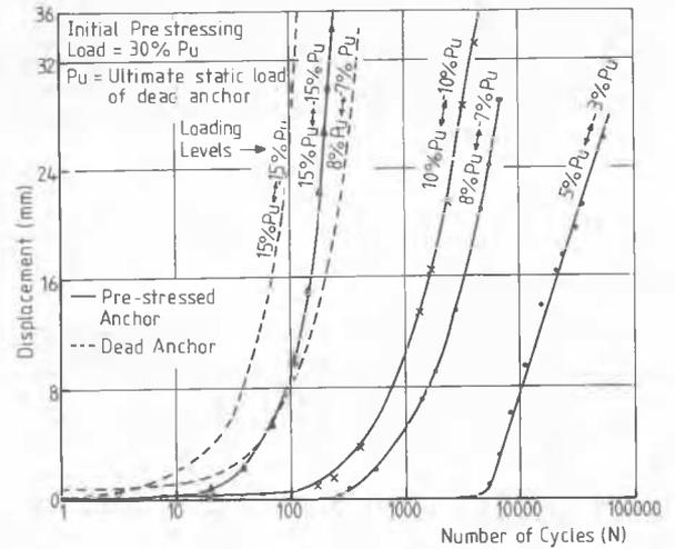
Figure 6. Displacement - log number of load cycles for anchors with initial prestress load of 30% Pu, compared with dead anchor performance - alternating loading.
