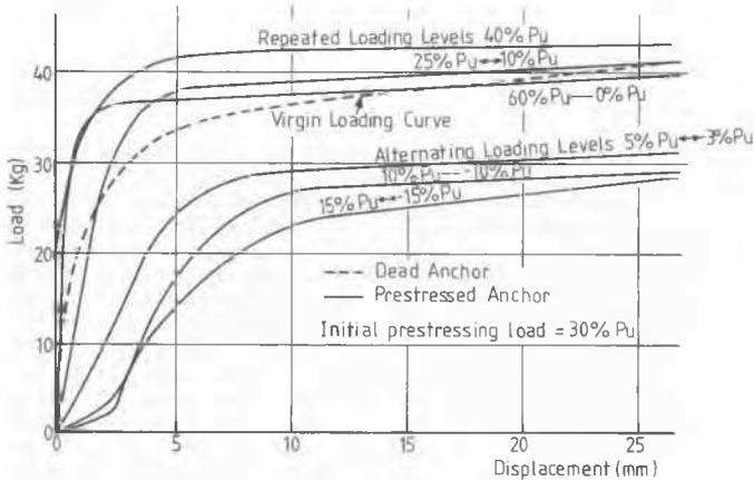
Figure 8. Effect of repeated and alternating loading on the static pull out resistance of anchors.
