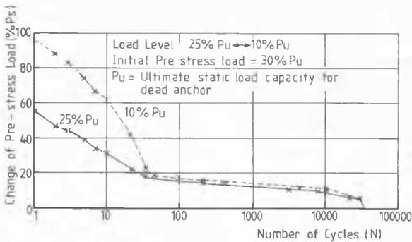
Figure 5. Loss of prestress load with number of load cycles - repeated load tests.
