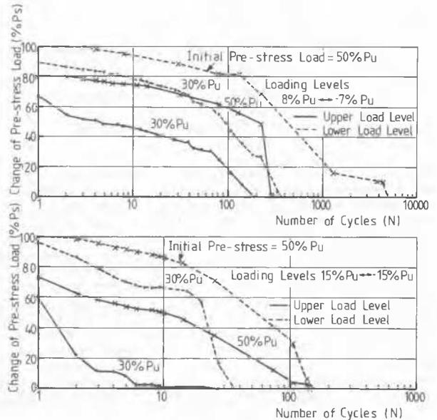
Figure 7. Loss of prestressed load with number of load cycles - alternating load tests.
