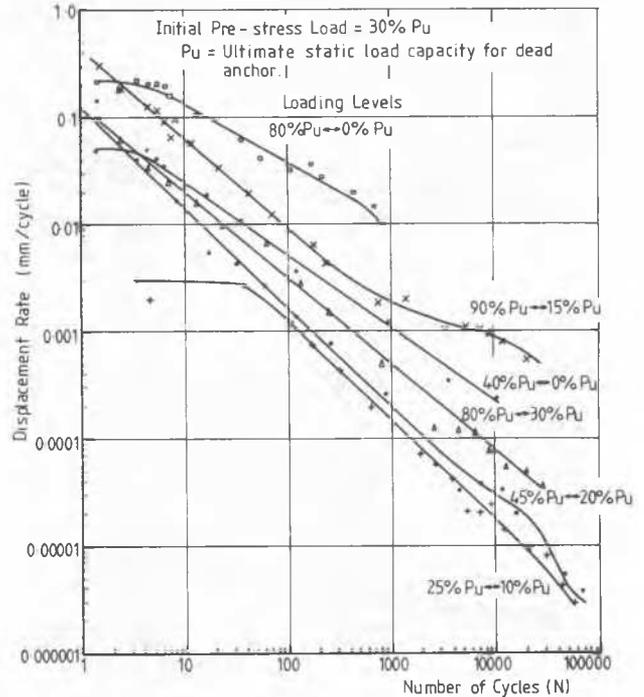
Figure 3. Rate of anchor displacement - number of load cycles relationship for anchors with an initial prestress load of 30% Pu.
