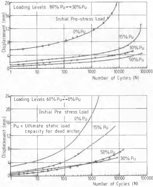
Figure 4. Displacement - log number of cycles for different values of initial prestress load.
