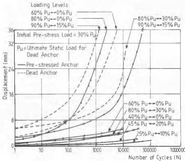
Figure 2. Displacement - log number of load cycles for anchor with initial prestress load of 30% Pu compared with dead anchor performance - repeated loading.
