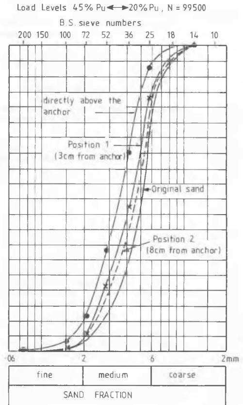
Figure 9. Grain size distribution of sand in the vicinity of anchor after a repeated loading test.
