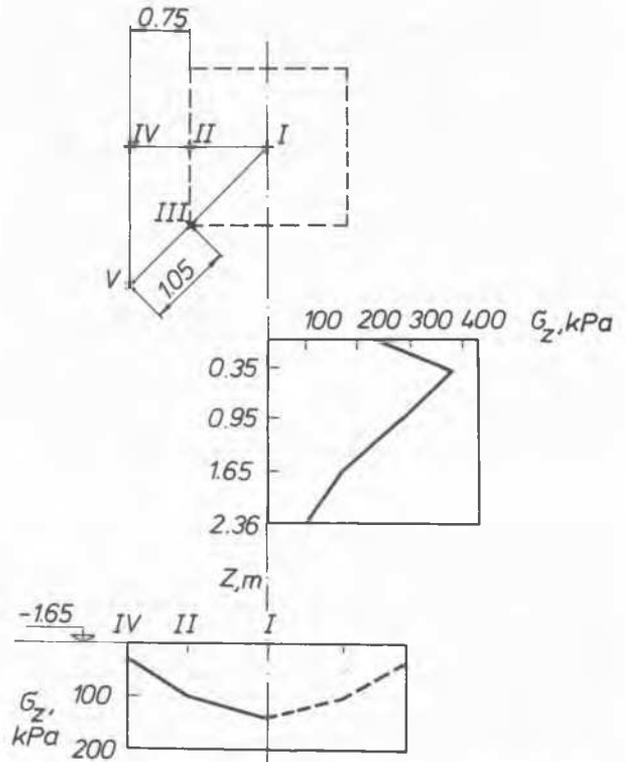
Fig.11 Vertical stresses under a plate with  $A=4 \text{ m}^2$ ; Site II,  $q=310 \text{ kPa}$
