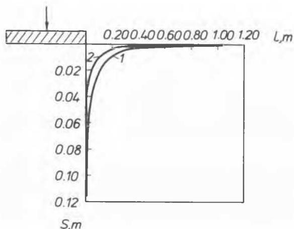
Fig.13 Distribution of deformations on the surface outside the plate ( $A=4 \text{ m}^2$ ), Site II
