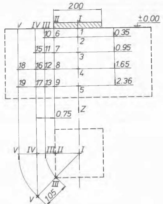
Fig.5 Position of earth pressure cells under the plate with  $A = 4 \text{ m}^2$ , Site II
