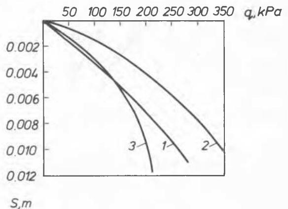
Fig. 12 Settlement-loading relationship, Site I, stabilized upper layer
