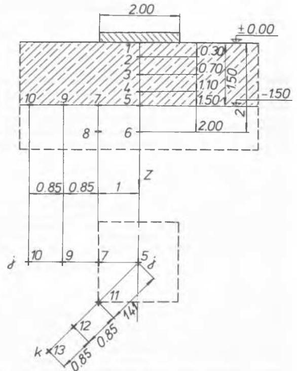
Fig.4 Position of earth pressure cells under the plate with  $A = 4 \text{ m}^2$ , Site I
