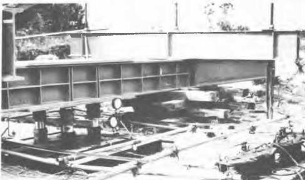
Fig.3 General view of the plate position on Site II,  $A = 4 \text{ m}^2$
