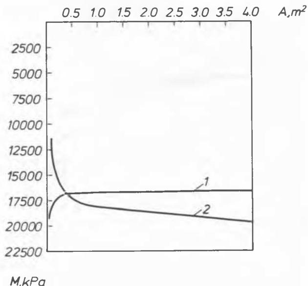
Fig.8 Modulus of deformation-plate area relationship
