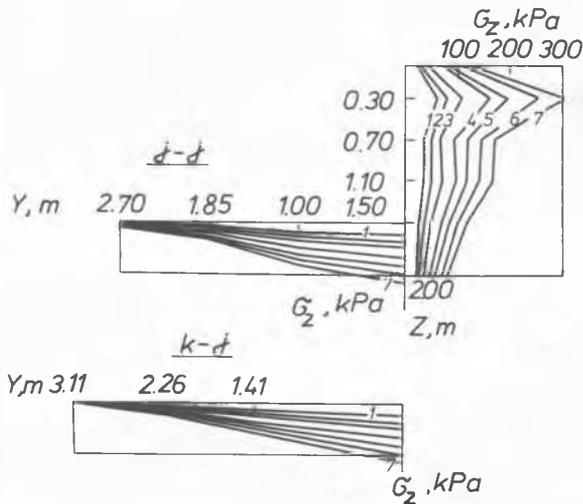
Fig. 10 Vertical stresses under a plate with  $A = 4 \text{ m}^2$ ; Site I
