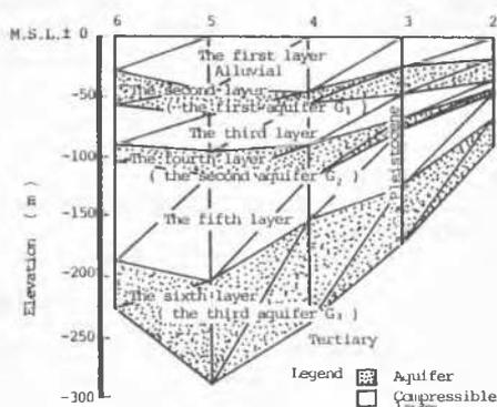
Fig. 5 West-east section of the model (M-M' section in Fig. 4)
