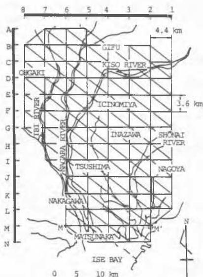
Fig. 4 Three-dimensional finite element model for the Nōbi plain
