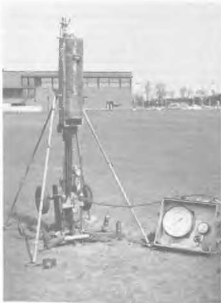
Fig. 5 Arrangement of the Borros AB static-dynamic penetrometer rig.
