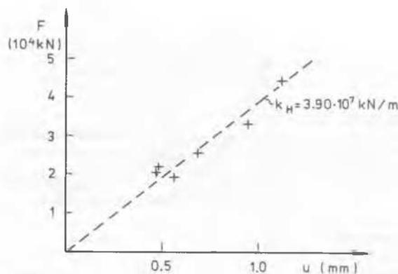
Fig. 3 Magnitude of horizontal base displacement vs. magnitude of horizontal force at sea bed.
