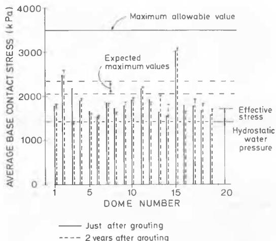
Fig. 6 Base contact stresses just after grouting and two years later.
