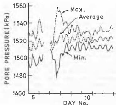
Fig. 5 Pore pressure in storm with significant wave height of 10.3 m during the first winter. Depth=4 m beneath sea floor.
