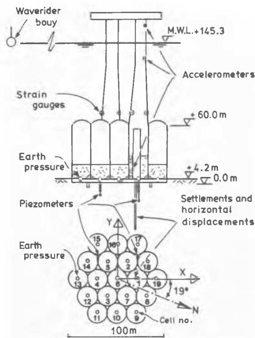
Fig. 1 Geometry of platform and location of sensors.
