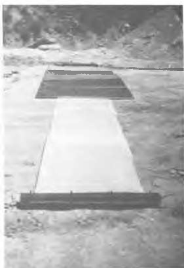
Fig. 3. - The flat jack covered by PVC. and steel plates
