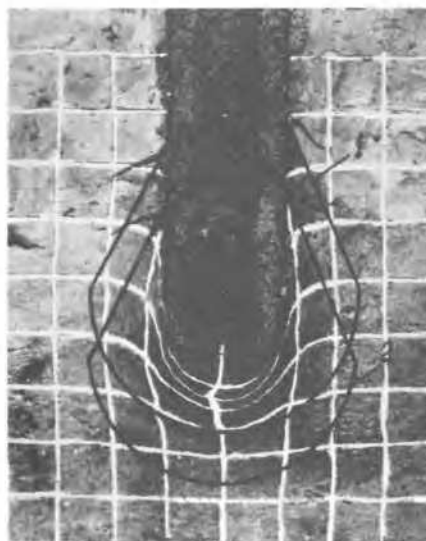
Fig. 1 Photo of successive failures traces in soil around the pile with two critical surfaces 1,2 plotted.
