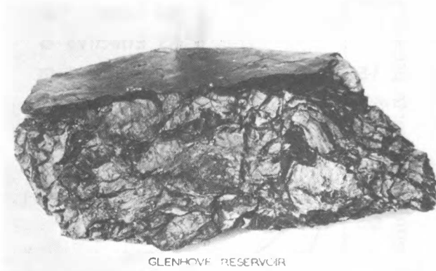
Fig. 5. SILTY CLAY FAILURE SURFACE
