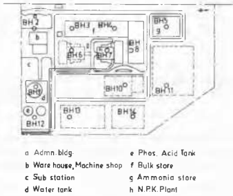
Fig 1a Plant layout & bore hole positions
