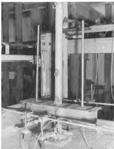
Fig. 1 Load apparatus for the model tests (without applying vertical loads)
