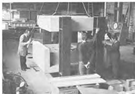
Fig. 5 Trial cell for testing the pressure cushions
