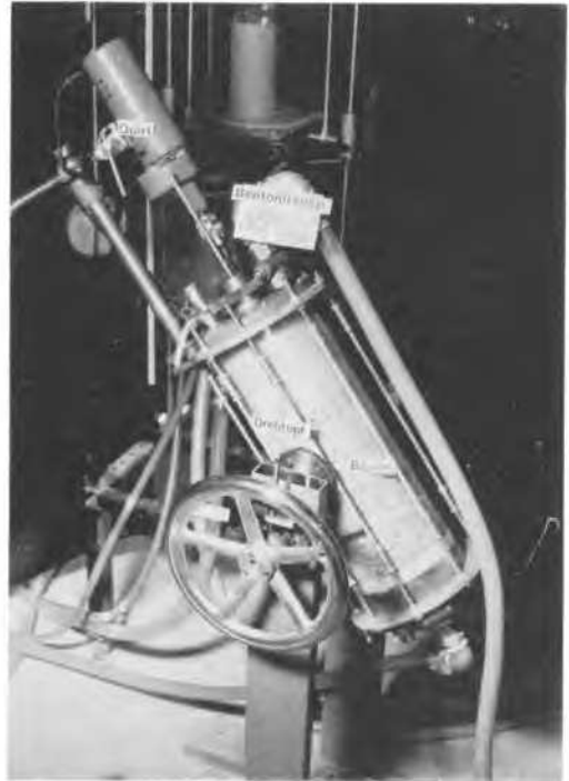
Fig. 9: Test apparatus for stability of inclined penetrated slopes
