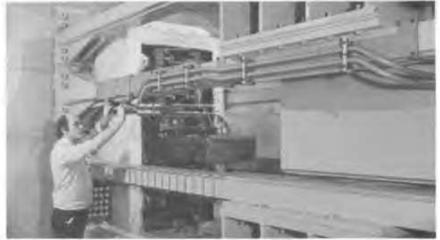
Fig. 2 Actuators mounted over model offshore platform
