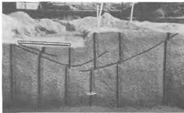
Fig. 6 Cross section showing lines of rupture beneath footing ( \delta = 20^\circ ) Test No. 2 in fill No. 2
