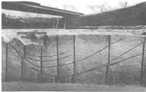
Fig. 5 Cross section showing lines of rupture beneath footing ( \delta = 10^\circ ) Test No. 3 in fill No. 2
