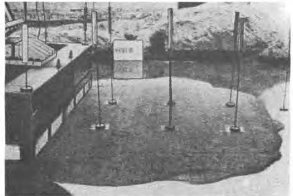
Fig. 3 Rupture line in front of one side of the footing ( \delta = 20^{\circ} ) Test No. 3 in fill No. 1
