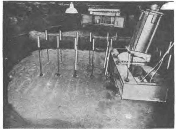
Fig. 2 Rupture line in front of one side of the footing ( \delta = 10^{\circ} ) Test No. 3 in fill No. 2
