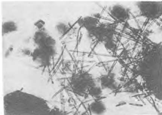
Fig. 2. - Electron micrograph showing prismatic gypsum forms, kaolinite, etc..
