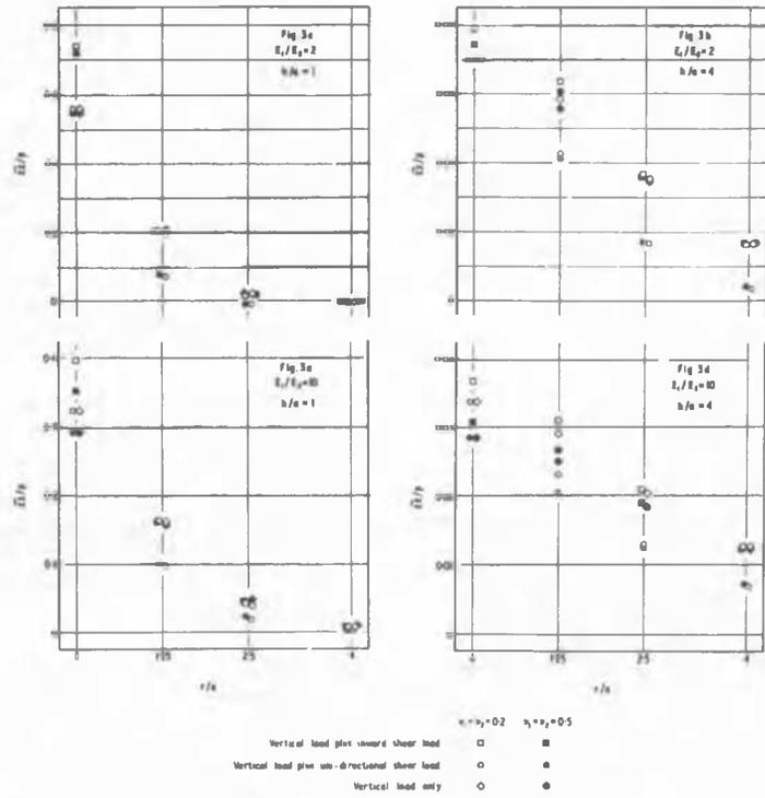
Fig.3. Vertical Direct Stress ( $\frac{zZ}{p}$ ) (at depth  $z = h$ ) vs. Radius ( $r/a$ )
