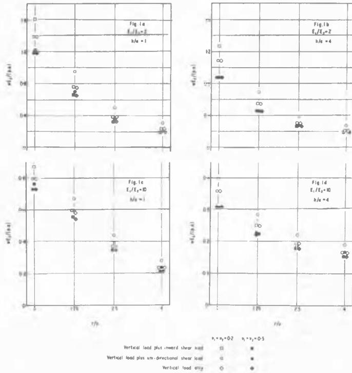
Fig.1. Vertical Displacement  $\left(\frac{w \cdot E_2}{p \cdot a}\right)$  (at depth  $z = 0$ ) vs. Radius ( $r/a$ )
