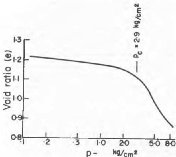
Figure 4 - The compression curve for Leda clay illustrating a high apparent preconsolidation pressure.
