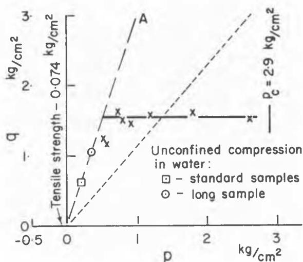
Figure 5 - A comparison of the results of indirect tension tests and unconfined compression tests in water with the compressive strength of Leda clay.
