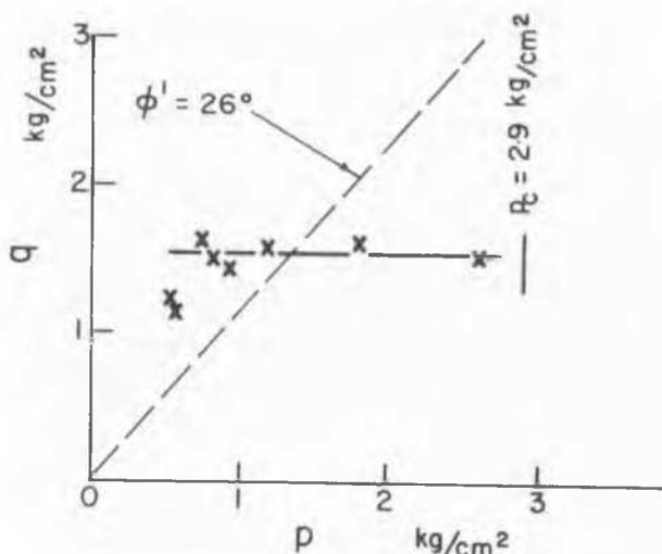
Figure 3 - The compressive strength of Leda clay.
