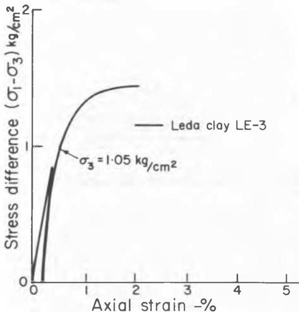
Figure 2 - Stress-strain behaviour in a cycle of loading for a naturally cemented soil.
