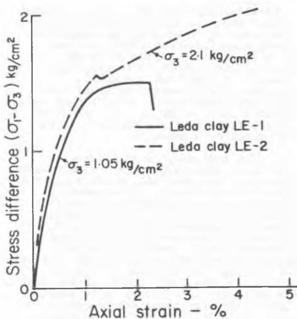
Figure 1 - Stress-strain behaviour for naturally cemented soils.
